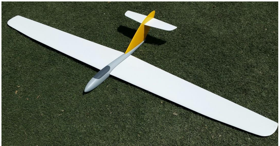
The Hybrid – F/G fuse, covered EPP wings and balsa tail feathers.
